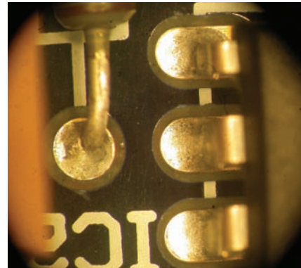
Close views of lead free PCB assemblies.
